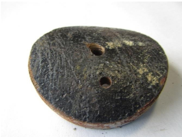
Figure 6.3-8 Exterior Surface of Lateral Coupon with Minor Pitting Corrosion
