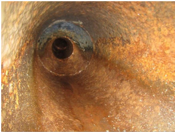
Photo 2-16. Dimple pattern (DI pipe); pitting and graphitization
