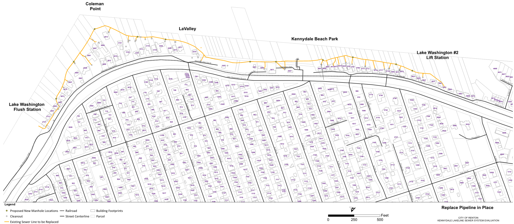
Figure 9.6 Replace-In-Place Lake Line Sewer Infrastructure
