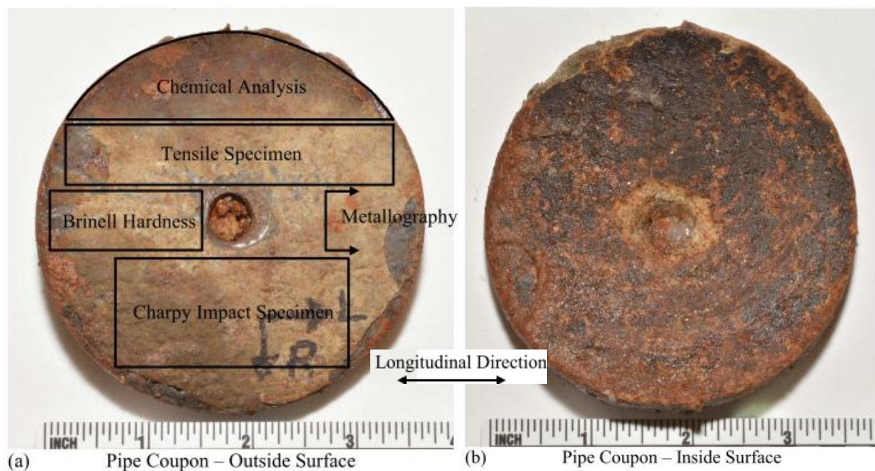
Figure 2-1. Pipe Coupon as Received by Laboratory
