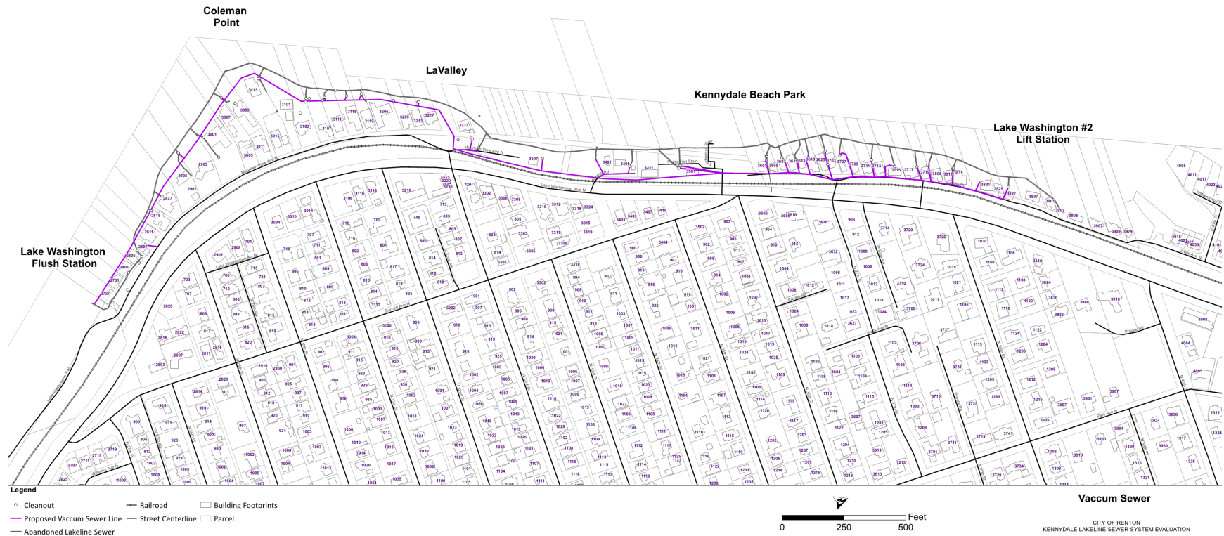
Figure 9.9 Vacuum Sewer Alternative Alignment
