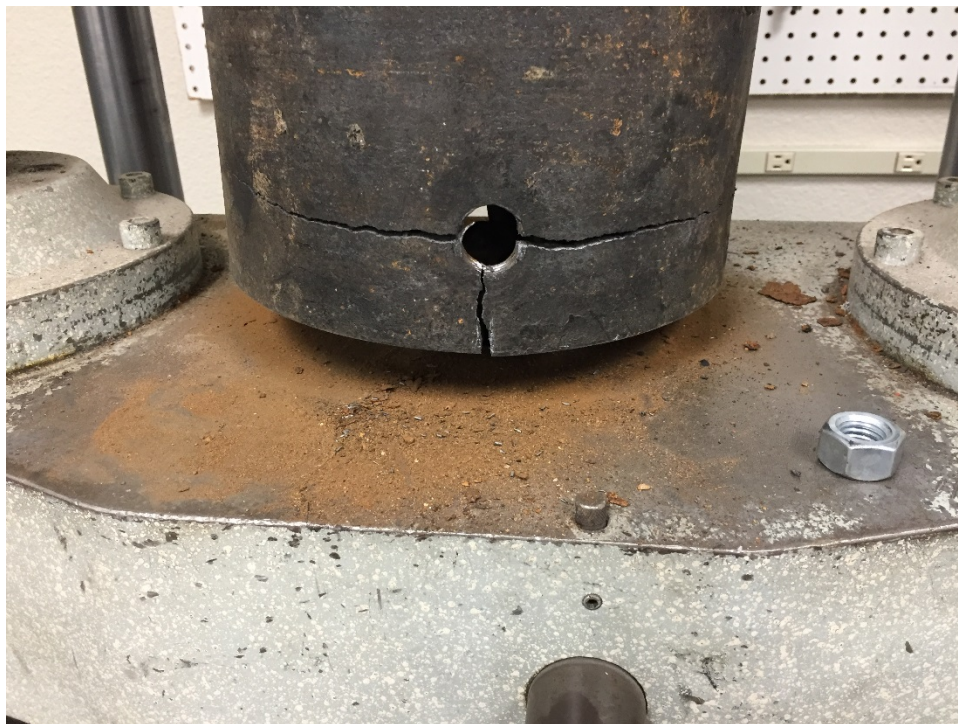
Photo #2 – Failure of pipe at connection bolt hole at 8,750 lbs.
