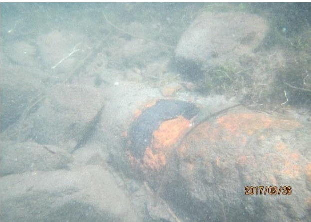
Figure 6.1-2 Area of Scaling and Tuberculation on Mainline; Large Rocks Around Mainline at 2811 Mountain View Avenue North
