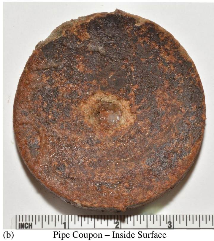
Figure 1 Photographs of the pipe coupon in the as-received condition (a) outside surface and (b) inside surface.
