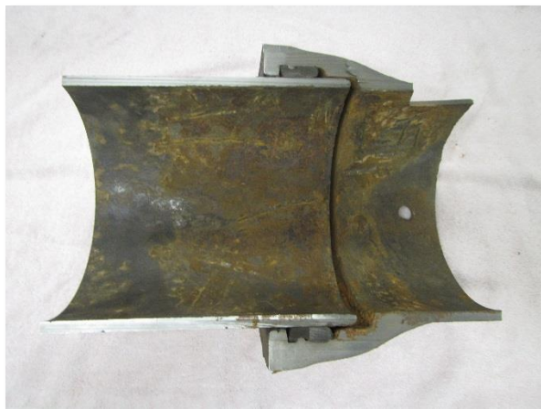
Photo 3-9. Manhole 5 Sample sectioned longitudinally to expose joint and rubber gasket.
