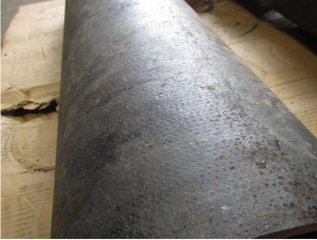
Figure 6.3-1 Typical Dimple Pattern on Mainline Samples and Coupon; However, this Is Cast Iron Pipe
