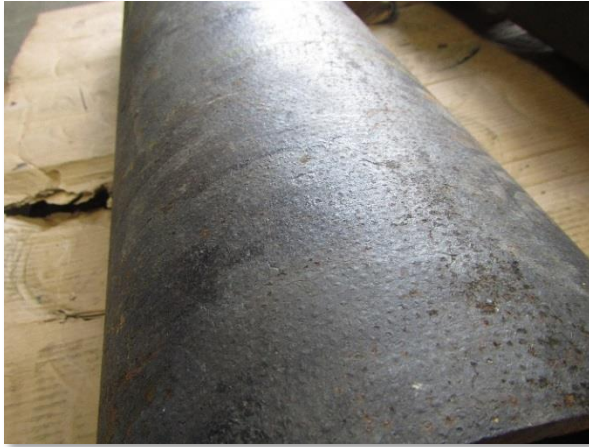
Photo 3-1. Typical dimple pattern on mainline samples and coupon; however, this is not ductile iron pipe.
